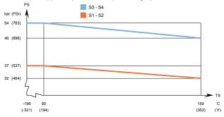
ACK74 - PED approval pressure/temperature graph
