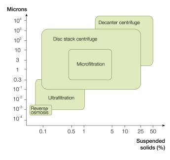
Alfa Laval offers separation equipment based on four complementing technologies:
